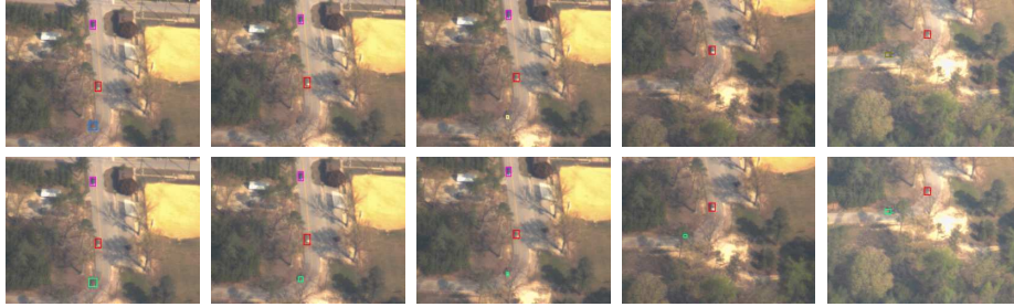
Fig. 4. Post linking result. Top: The ID of blue car has been changed several times due to occlusion by trees. Bottom: The car’s ID is maintained after linking process.
