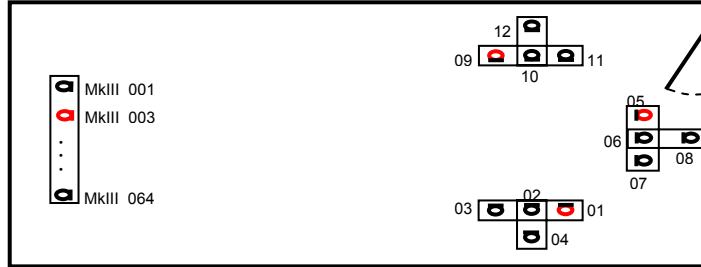
Figure 4. The choice of the microphones for the UPC smart-room
