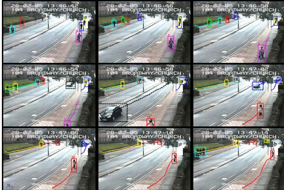
Fig. 2. Typical frames from the outdoor recordings with the tracked targets superimposed. Dashed bounding boxes and lines correspond to vehicles and their tracks.
