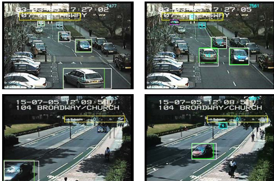
Fig. 2. Results of vehicle tracking and detection (Yellow box: DCO (Dont Care Object), Green box: Detected ground truth, White box: Detected system output, Blue box: Missed ground truth, Black box: Detected but overlapped with DCO, Magenta box: Occluded ground truth (DCO), Cyan box: Stationary ground truth (DCO))
